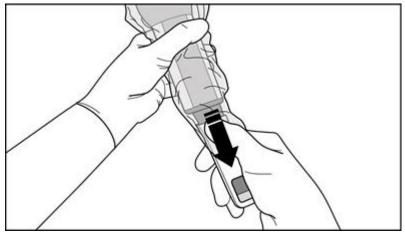
Figure 121: Slightly release the rigid section of the wand barrier sleeve from the tip of the wand
