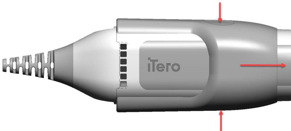
Figure 148: Release and remove the vent cover
