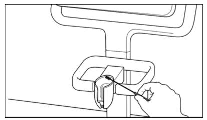
Figure 153: Remove remaining marks and stains on the cradle using the soft bristle brush
