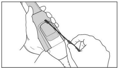
Figure 146: Remove marks and stains using a soft bristle brush
