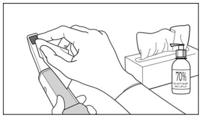
Figure 147: Wipe the optical surface of the wand with IPA
