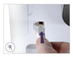
17. Connect the wand cable to the back of the touch screen.
