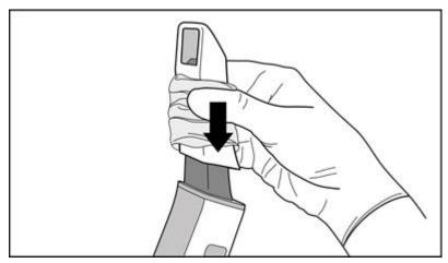
Figure 57: Slide the rigid section of the wand barrier sleeve into place
