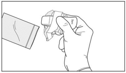
Figure 56: Remove the wand barrier sleeve from its packaging
