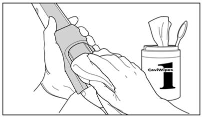
Figure 145: Remove gross contaminants using CaviWipes1
