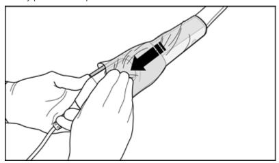
Figure 58: Gently pull the transparent sheath to cover the entire wand
