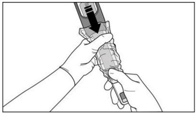
Figure 120: Scrunch the transparent sheath halfway towards the tip
