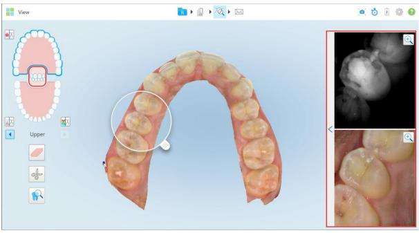
Figure 105: Viewfinder on the right showing the area in the loupe in both NIRI and color modes
