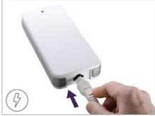
2. Connect the hub power cable to the hub.
