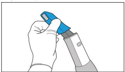
Figure 55: Remove the protective sleeve
