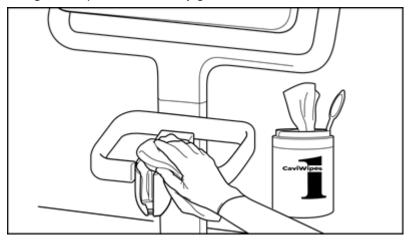
Figure 152: Remove gross contaminants on the cradle using CaviWipes1
