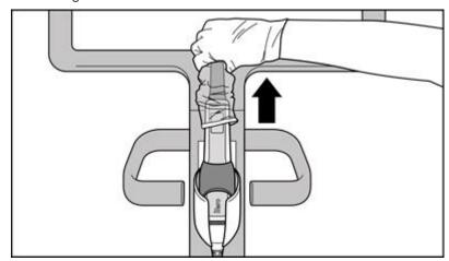
Figure 122: Remove the wand barrier sleeve
