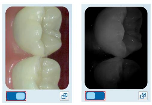
Figure 77: Viewfinder displaying a color image (left) or a NIRI image (right)
